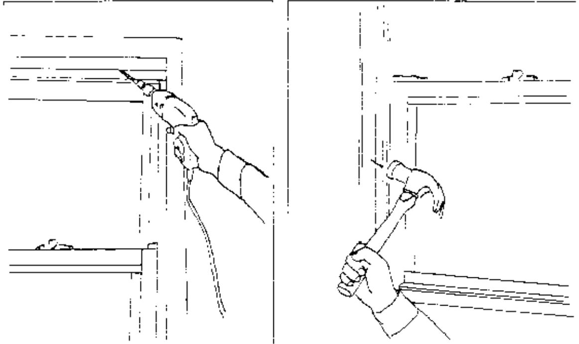
Adjust top expander all the way up if necessary. Caulk around the entire perimeter of the window on the outside, then inside. Replace the old trim strips or install new trim at the head and jambs
