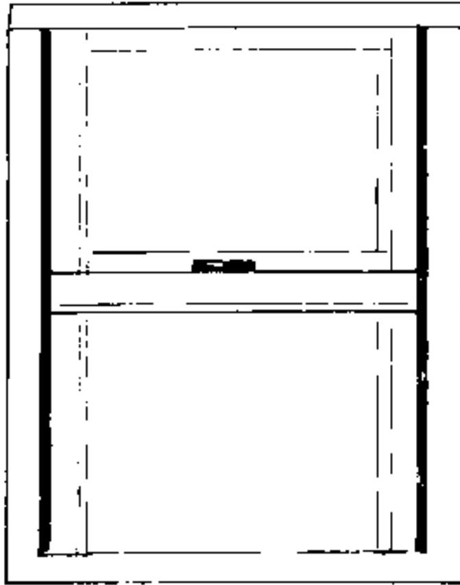
Sash gap should be the same at the mid section of the window as it is at the top and bottom
